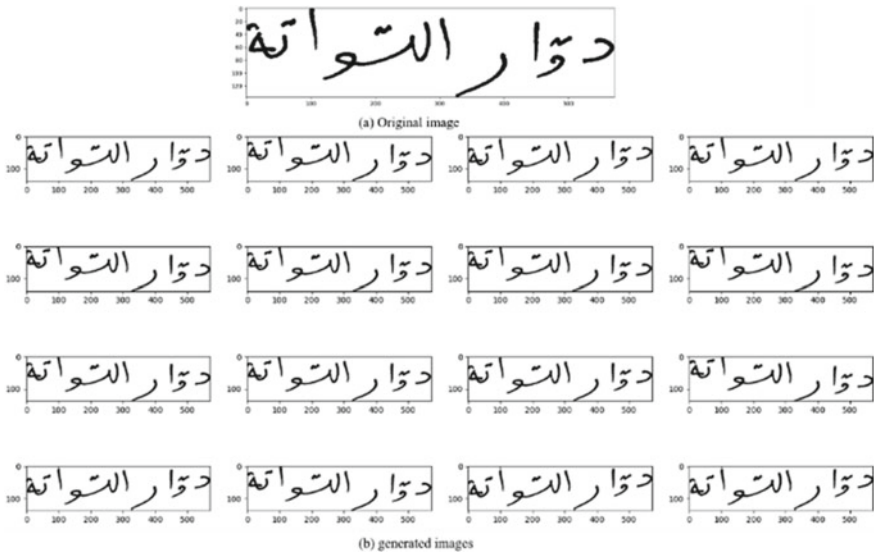
Fig. 1 Image augmentation using image data generator from Keras library of Tensorflow, a original image, b fifteen randomly generated images: rotation up to 2^\circ , width and hight shift up to 2, shearing up to 4
