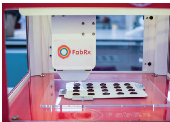
Fig. 7.2 3D printing technique (semi-solid extrusion) to make chewable drugs [9]
