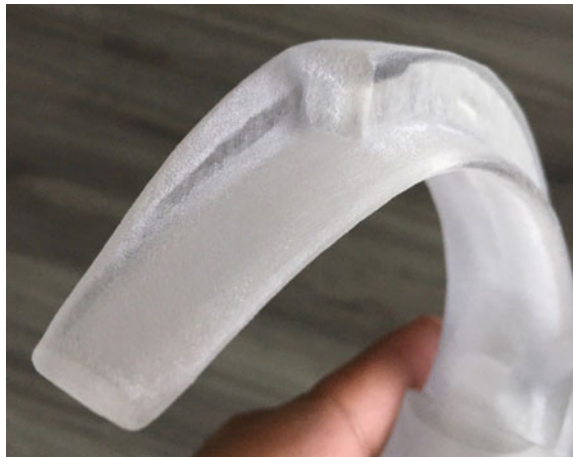
Fig. 3 The tip of a 3D printed laryngoscope blade with the expected location of the camera window. Note the lack of window transparency
