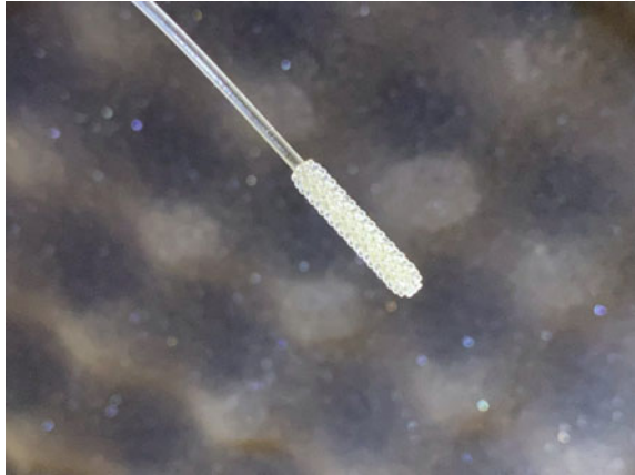
Fig. 7 Close-up of the 3D printed testing Swab ( https://www.materialise.com/en/hands-freedor-opener/technical-information )
