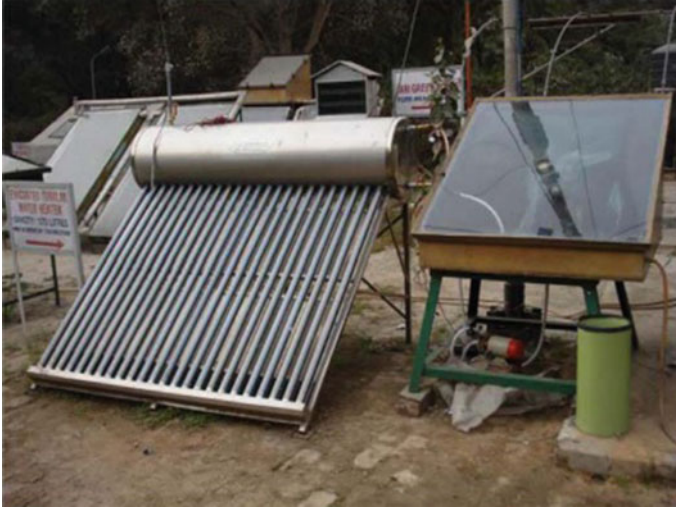
Fig. 7 Solar still assisted ETC heat chamber [33]
