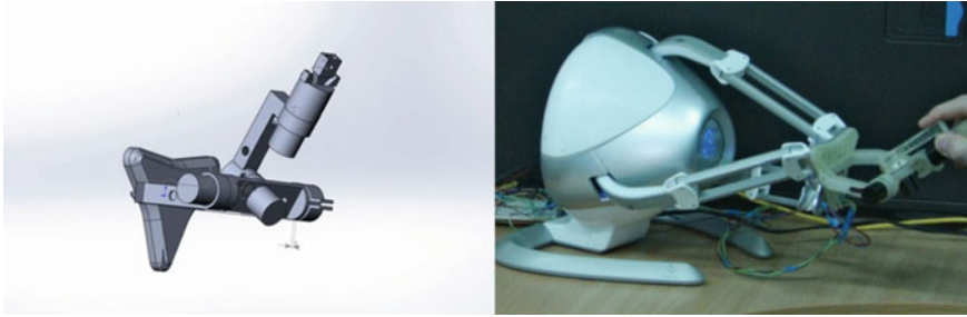
Fig. 10 Custom-designed grip to provide extra three-degrees of freedom
