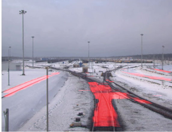
Fig. 5 Image frame with a mask obtained after execution of the morphological closure
