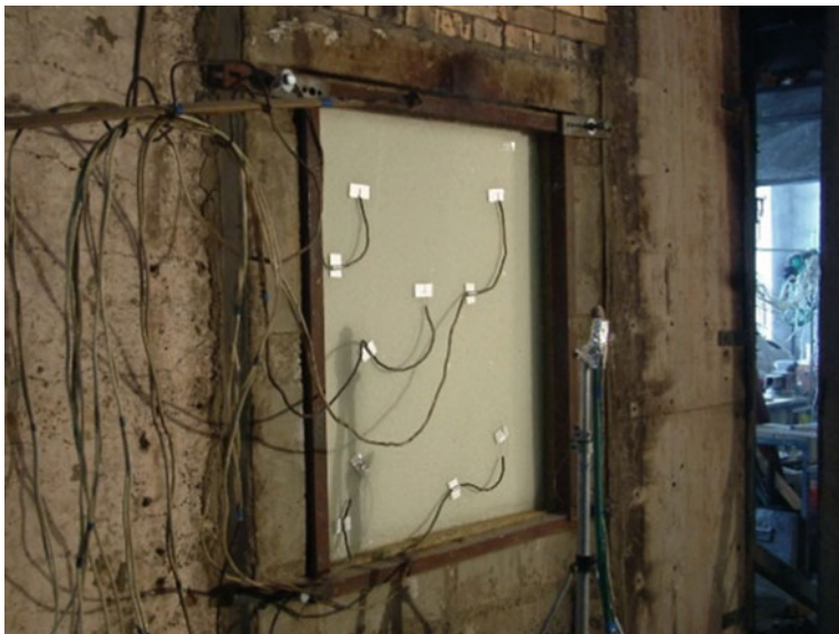
Fig. 13 Tests of fire-resistant glass Brand Glass Paraflam, 1200 × 1000 × 28 mm, EIW 60
