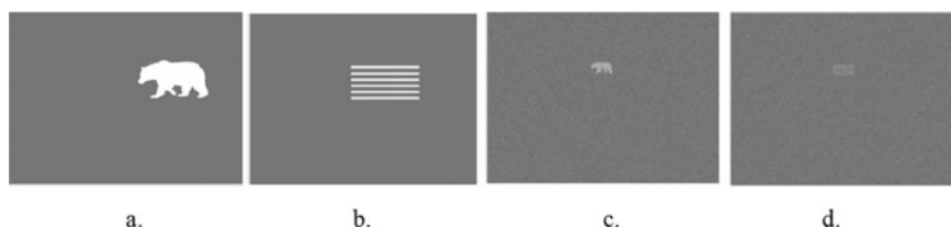
Fig. 5 An ideal input signal and the output image without processing: a typical ideal object; b equivalent ideal bar; c the output image of typical object without processing; d the equivalent bar of typical object without processing
