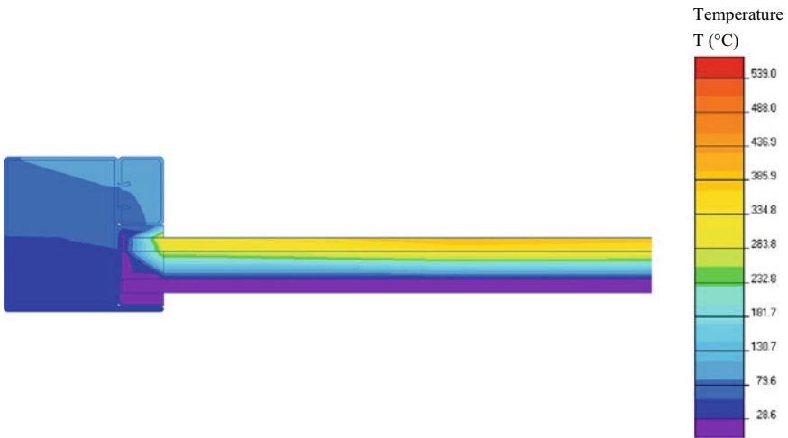
Fig. 7 Temperature field of a two-chamber double-glazed window with tempered glass after 3 min
