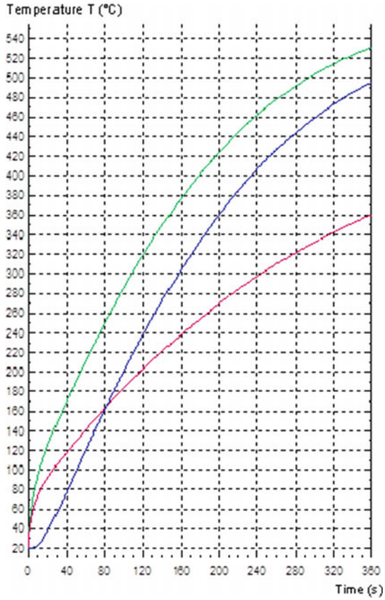
Fig. 9 Growth curve of temperature in time for a single-chamber double-glazed window with tempered glass
