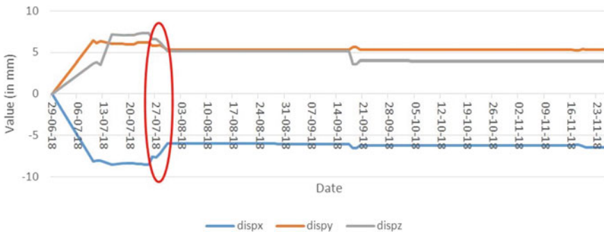
Fig. 6 Movement recorded by LMWS in X-, Y- and Z-direction between 29 June 2018 and 23 November 2018. The movement due to the flash flood at Paddhar on 27 July 2018 has been highlighted with a red oval
