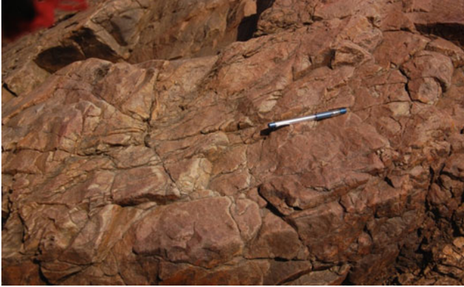
Fig. 2 Mosaic texture in quartzitic sandstone
