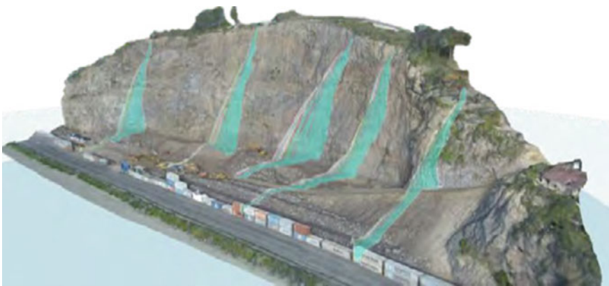
Fig. 3 2D rockfall analysis undertaken on cross section re-imported back into the 3D (after Rose et al. 2008)
