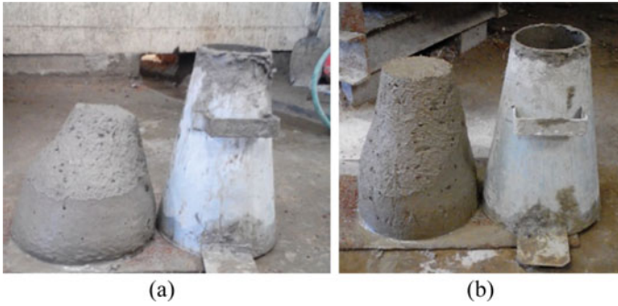
Fig. 3 True slump of coconut shell concrete a Without fibre, b with fibre
