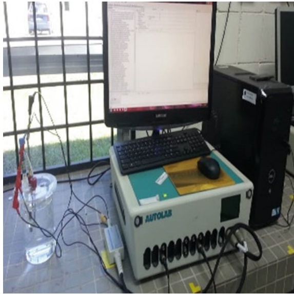
Fig. 3 LPR setup with ACM software
