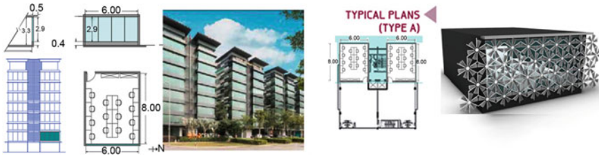
Fig. 5 Star Central Typical plan A and office space proportions
