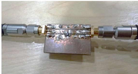
Fig. 9 Test board B measurement of pin 1 and pin 6 through CPWG transmission line with SMA connectors
