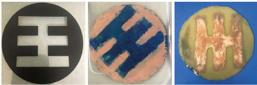
Fig. 5 Patterning mask (left); Copper board after development (mid); copper board after etching (right)
