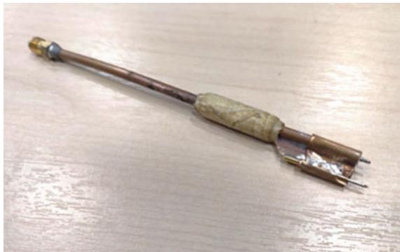
Fig. 4 A low cost coaxial probe with a pogo pin soldered to the ground
