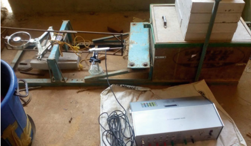
Fig. 1 Pullout test setup
