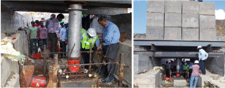
Fig. 5 Photograph of test set-up for shear
