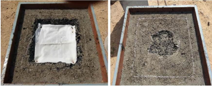
Fig. 7 Pothole simulation with and without geotextile layer
