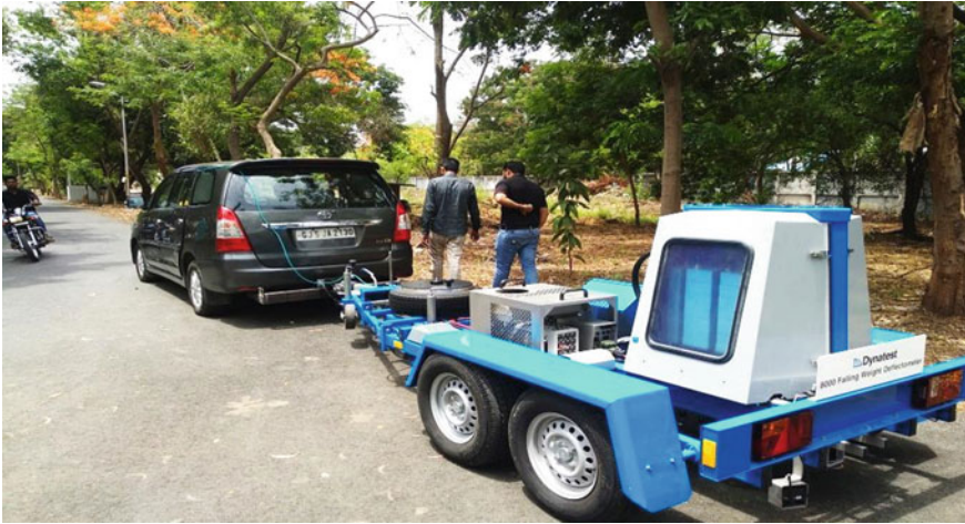
Fig. 4 DYNATEST falling weight deflectometer (FWD)
