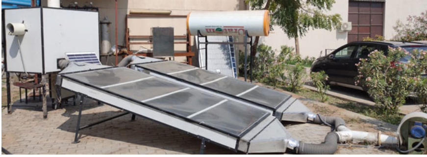
Fig. 13.6 Solar drying setup with PCM storage at Pandit Deendayal Petroleum University ( Source Author )
