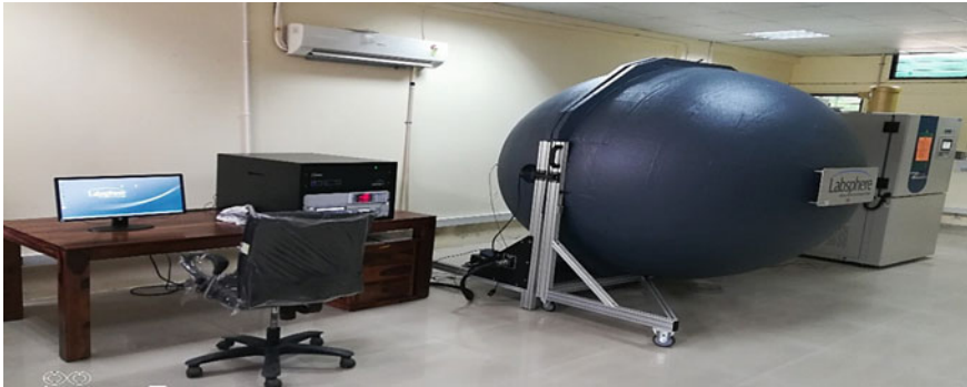
Fig. 8.19 Integrating sphere with temperature-controlled system. Source Author
