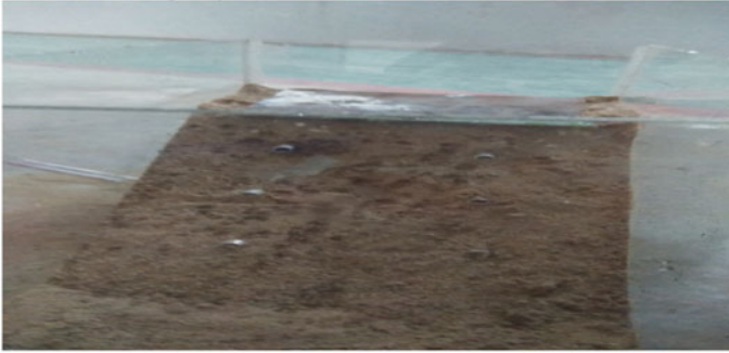
Fig. 1 Model box with 45° soils and with nails for test
