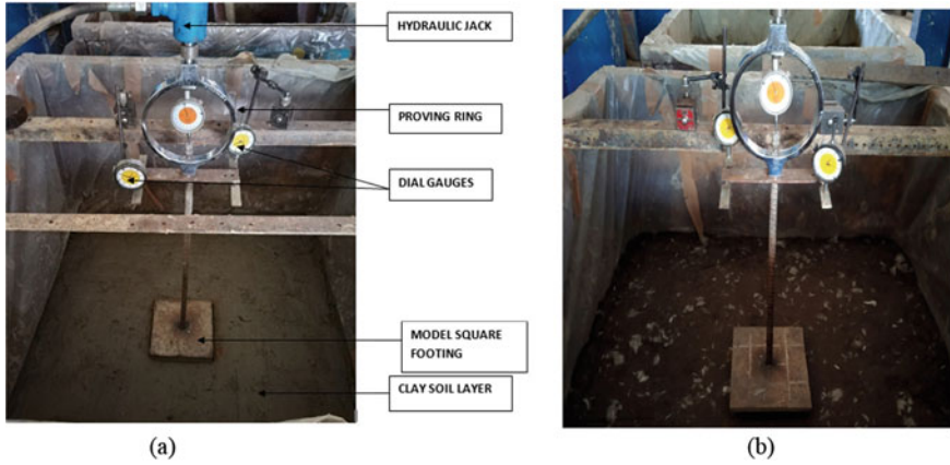
Fig. 3 a Model tank with loading arrangement on soft clay layer, b placing the cement modified fibre reinforced sand layer on top of soft clay layer
