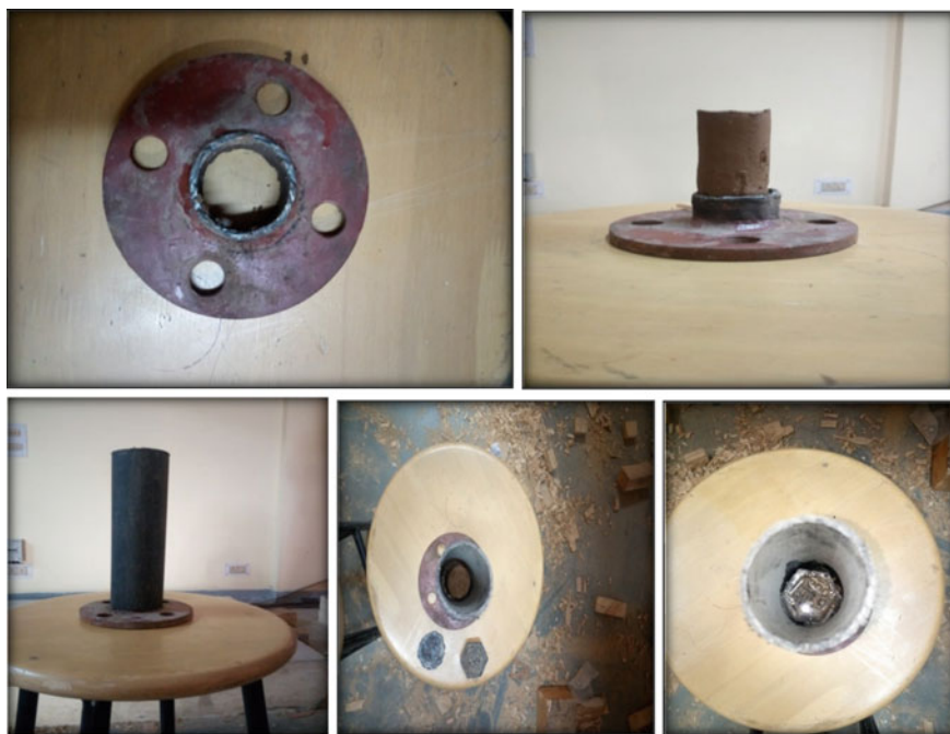
Fig. 2 Mould and sample preparation for curing stress
