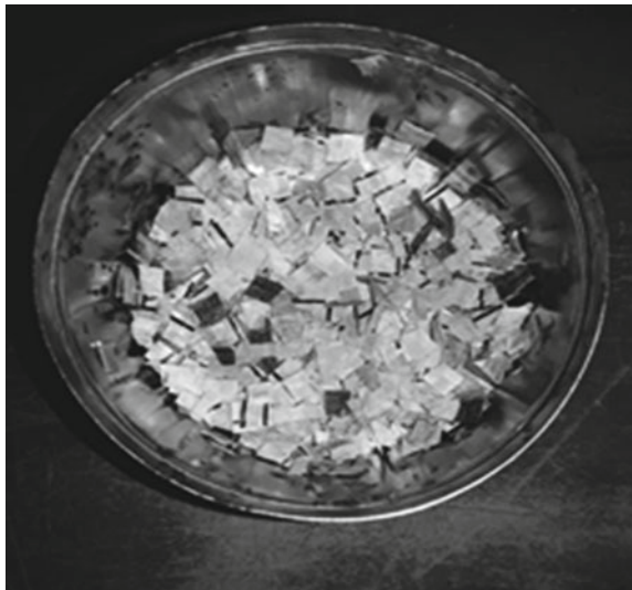
Fig. 3 Used cut pieces from cement bag
