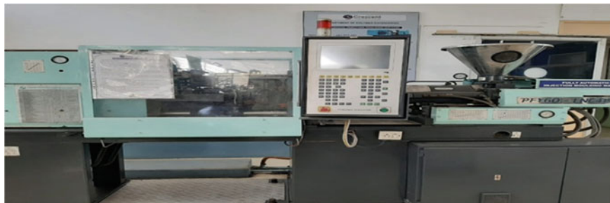
Fig. 1 Injection molding machine to prepare the samples as per ASTM standards
