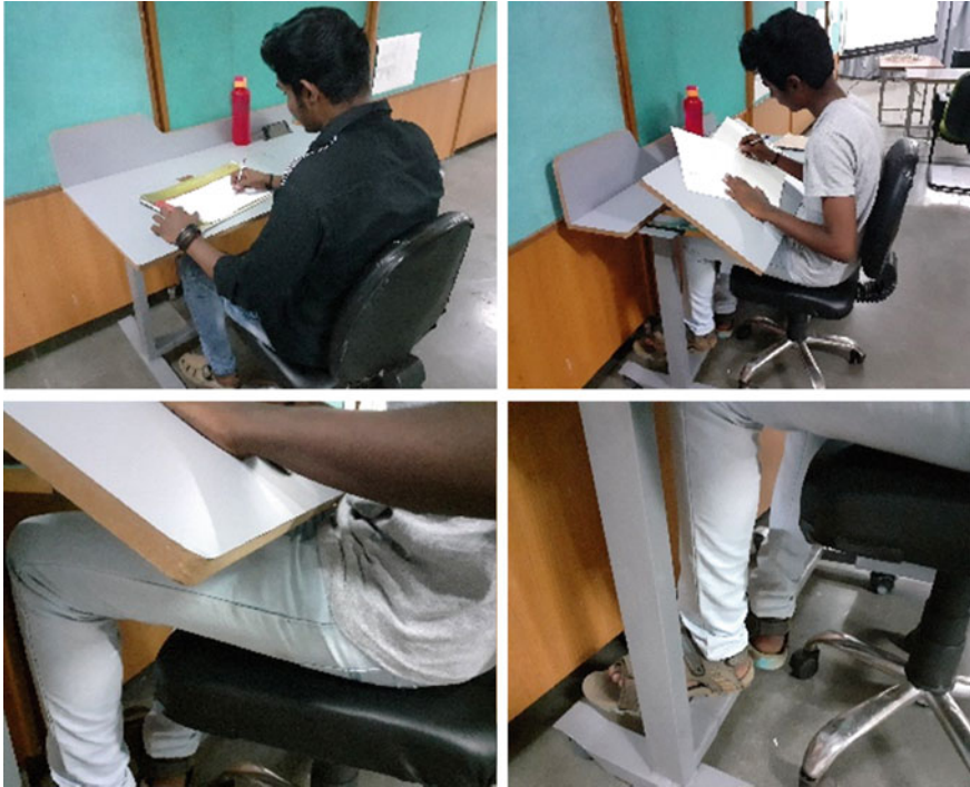
Fig. 7 Final products' ergonomic and usability testing with the users
