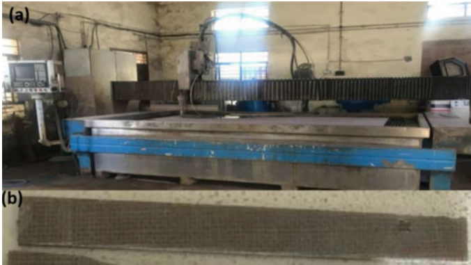
Fig. 3 a Waterjet machine, b cut sample of hybrid polymer composite
