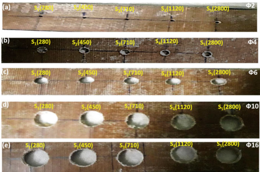
Fig. 7 Macroscopic images of drilled holes in hybrid polymer composite for different diameter of drill tool. a 2 mm, b 4 mm, c 6 mm, d 10 mm, e 16 mm
