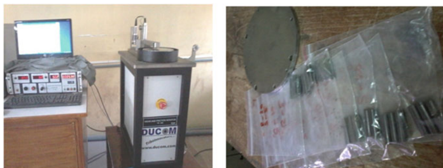
Fig. 1 Ducom wear and friction tester with data acquisition and specimen tested
