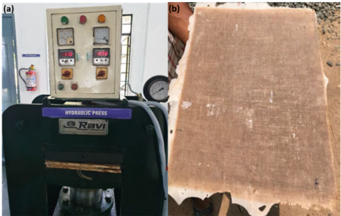
Fig. 2 a Hydraulic press, b prepared composite
