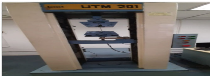
Fig. 2 Universal testing machine to conduct tensile tests of samples
