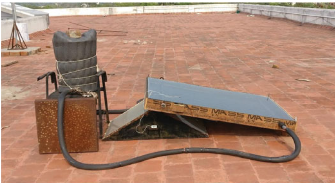
Fig. 1 Experimental setup of solar water heater
