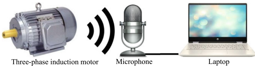
Fig. 1 The sound recording/monitoring system
