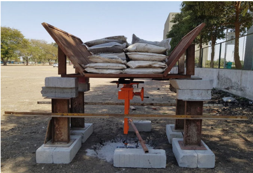
Fig. 7 Plate load test using geo-cell
