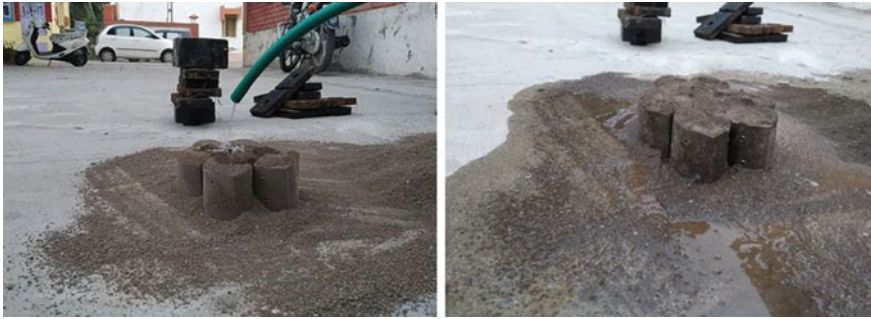
Fig. 5 Drainage test of geo-cell (left full saturation, right free drainage of water)
