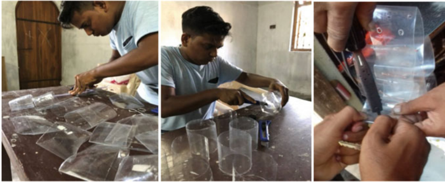
Fig. 1 Preparation of geo-cell from plastic bottles (cutting, joining, and perforations)
