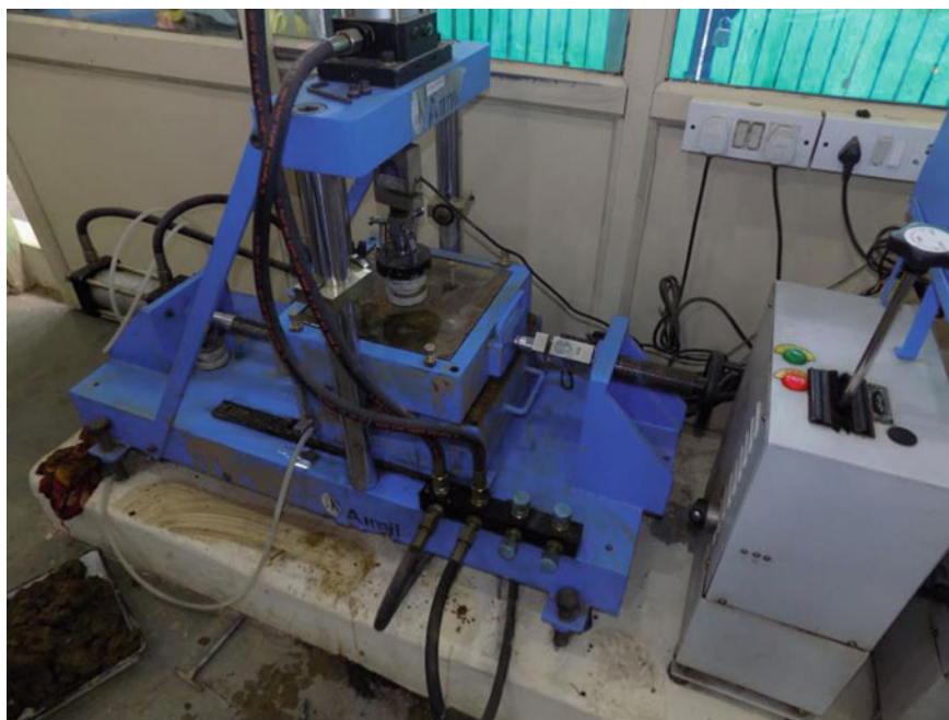
Fig. 1 Large-box direct shear test apparatus, Aimil make
