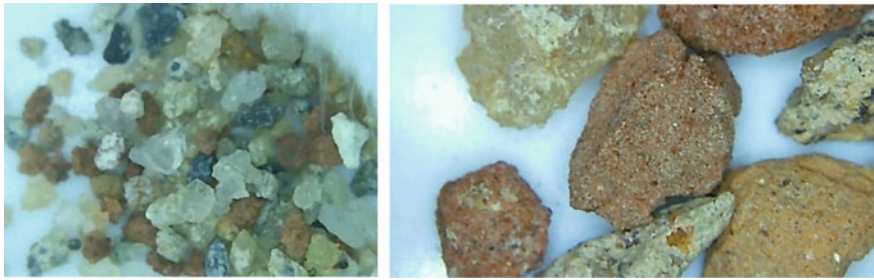
Fig. 2 Grains shape of MRA from two processing plants at 50X magnification
