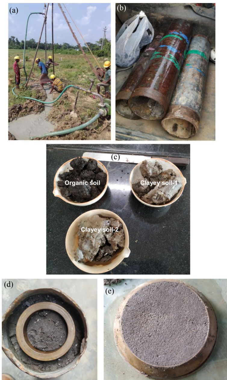
Fig. 3 a Extraction of sample from site. b Thin tube soil samplers. c Three types of soil samples. d Consolidation ring in sampler. e Soil sample for consolidation. f Extraction of soil sample from sampler for triaxial test. g Soil collected in small D samplers. h Samples for CU triaxial test
