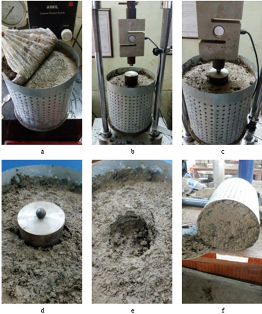
Fig. 6 Testing procedure a Removing top cover after soaked for 96 h, b Placing mould under loading frame along with footing at centre, c Applying point load to the footing, d Footing after testing, e Settlement of the footing, f Removing sample from the mould
