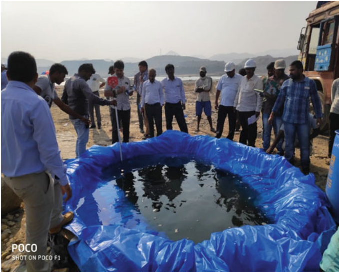
Fig. 3 Determination of in-situ density of rockfill material using water replacement method
