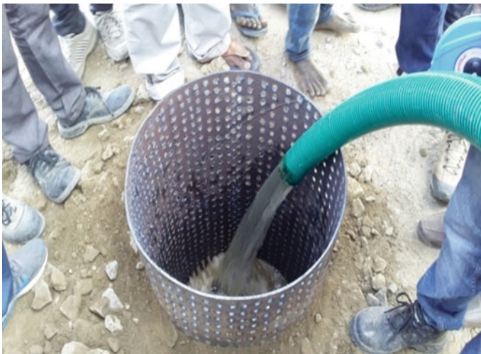
Fig. 4 Field permeability test to determine field permeability of rockfill material
