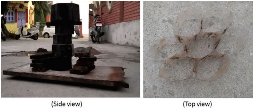
Fig. 4 Static compressive strength test of plastic waste geocell(right-loaded, left specimen)
