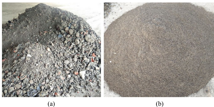
Fig. 2 a Stockpile of MSWI bottom ash and b soil-like fraction from MSWI bottom ash
