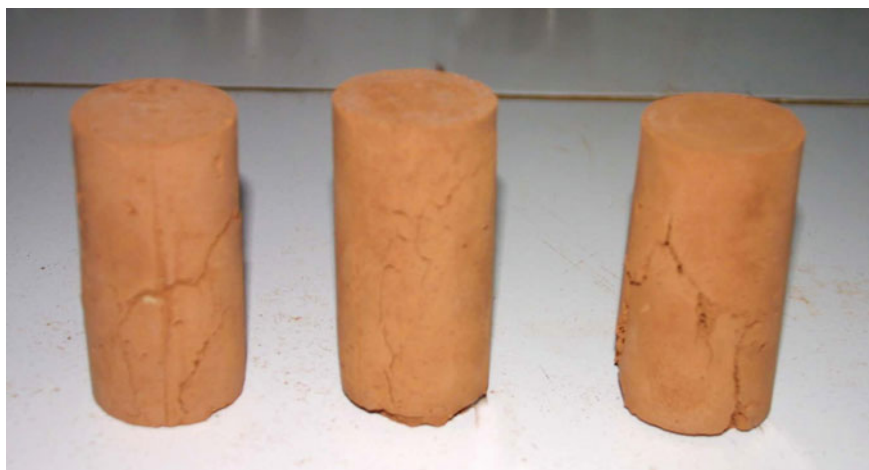
Fig. 2 Failure pattern of cement stabilized sample by UCS test
