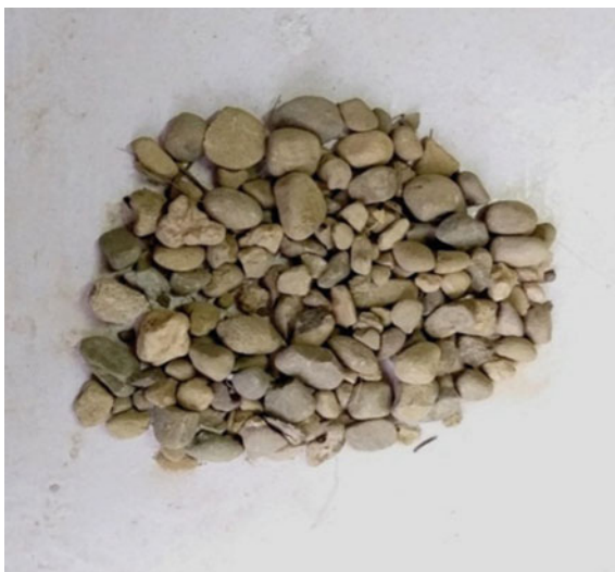
Fig. 4 Granular material of size 8 to 10 mm
