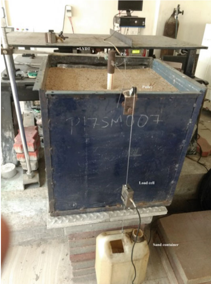
Fig. 5 Test arrangement after cyclic loading
