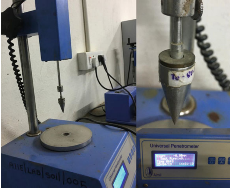
Fig. 4 Cone penetrometer apparatus used in testing
