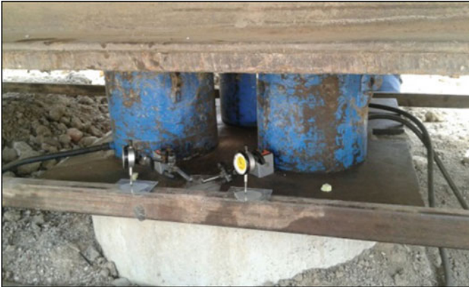
Photograph 3 Jacks and dial gauges in load test
