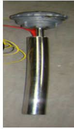
Fig. 3 Modified thermocouple controlled heater rod
