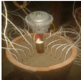
Fig. 3 Modified thermocouple controlled heater rod
