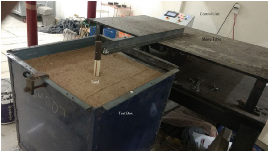
Fig. 4 Cyclic loading test arrangement with connections
