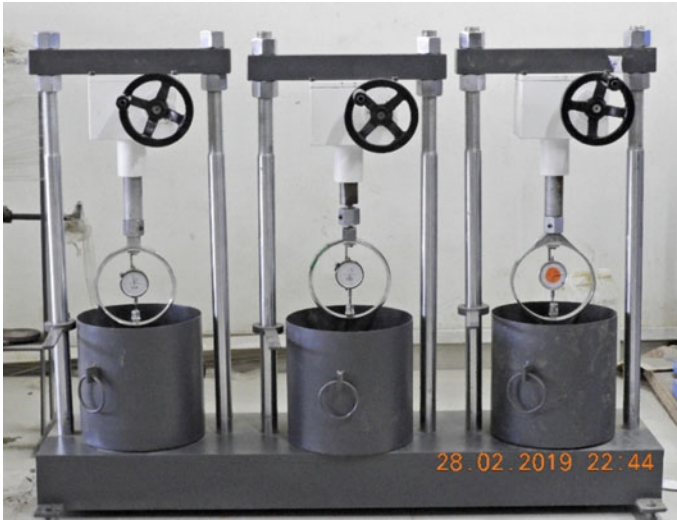
Fig. 2 Swelling test on soil using apparatus
