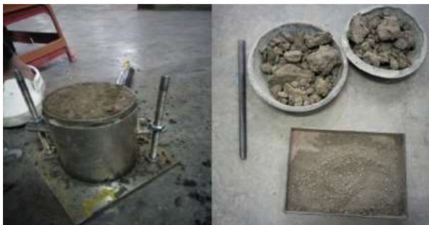
Fig. 3 Proctor compaction test setup
