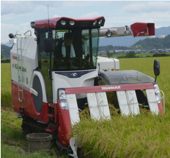
Fig. 9 Rice harvest using a smart combine harvester in a large-scale farm of Kinki Region, Japan (Source Photograph by the authors)
