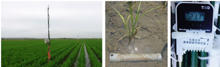
Fig. 10 Paddy sensor and meteorological sensor for precision irrigation
