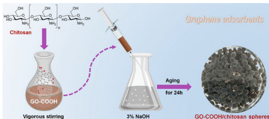
Fig. 9 Schematic illustrations of the synthesis process of GO-COOH/CS spheres for Cu 2+ fixation. Reproduced with permission from [38]
