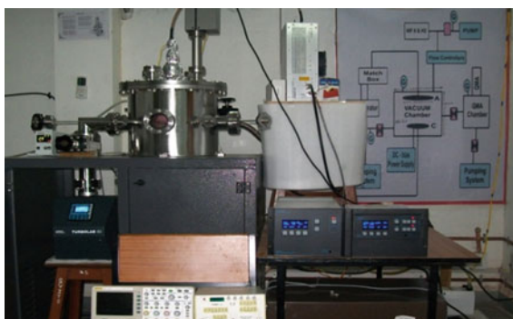
Fig. 3 Schematic of the RF plasma treatment reactor at SVVV
