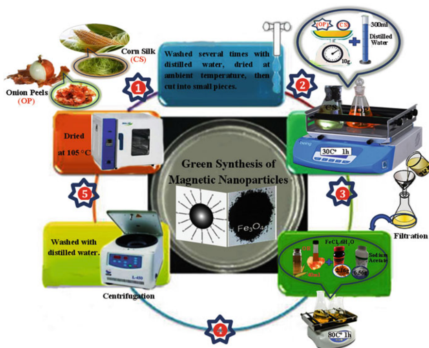
Fig. 9.6 Synthesis of green magnetic nanoparticles
