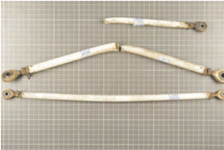
Fig. 5 Bending and rupture of connecting rod
