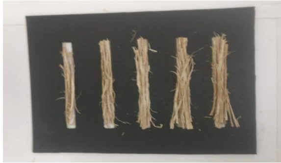
Fig. 3 Fibers organized according to given volume fractions
