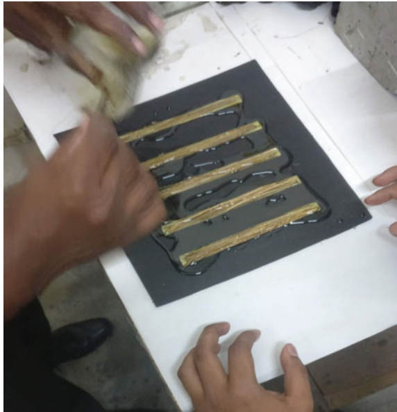
Fig. 4 Resin mix is being poured over the fiber molds
