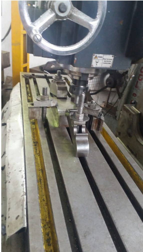
Fig. 3 Fixture developed for FSW process
