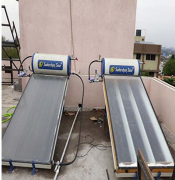
Fig. 2 Simple solar water heater and solar water heater with V-trough reflector
