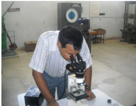
Fig. 2 Measurement of bead dimensions
