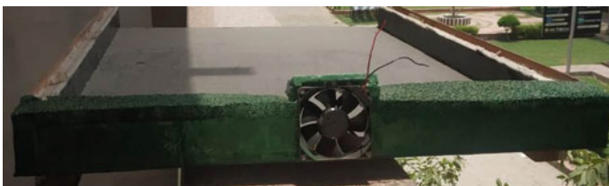
Fig. 2 Duct incorporated with DC fan in PVT system
