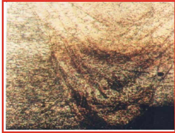
Fig. 1 Measurement of penetration depth and bead length by image analyzer
