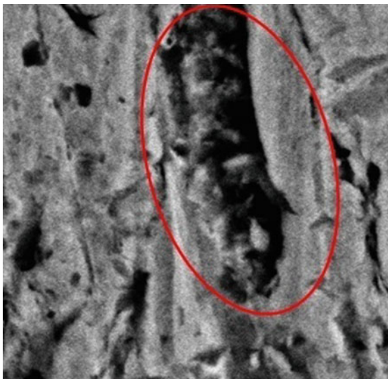
Fig. 4 SEM image of crack in Cu-Al 2 O 3 -C hybrid MMC
