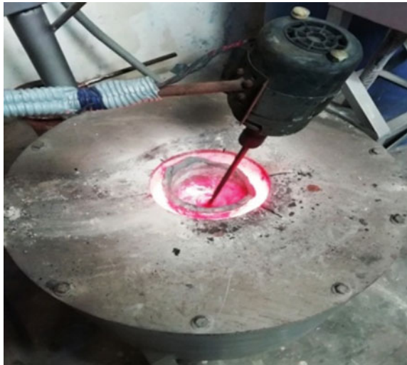
Fig. 4 Motorized stirring of HMMC
