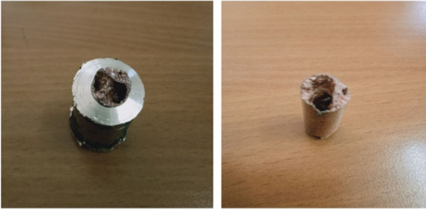
Fig. 2 Porous Cu-ZrO 2 -C composite formed by stir casting
