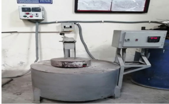
Fig. 1 Electric furnace (up to 1400 °C)
