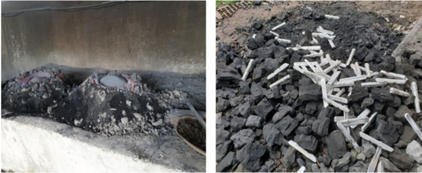
Fig. 4 Dross in aluminium waste [8]
