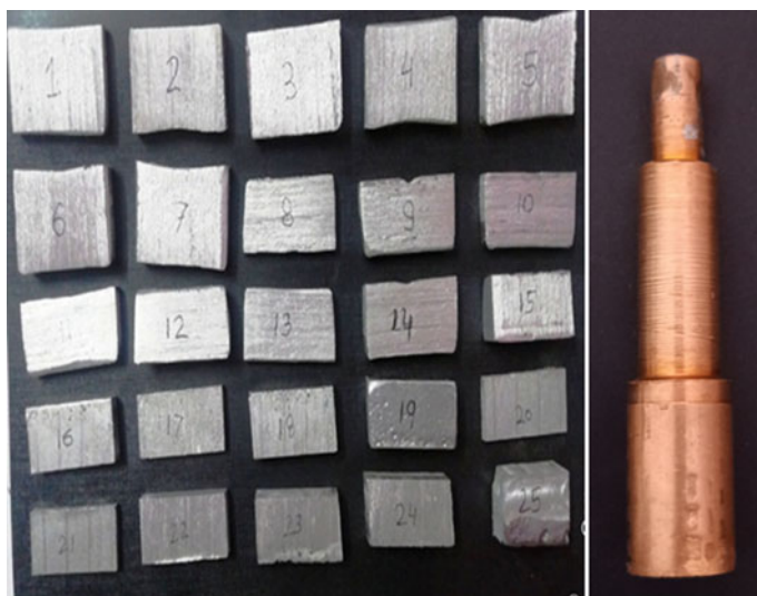
Fig. 1 Prepared composite samples with copper cutting tool
