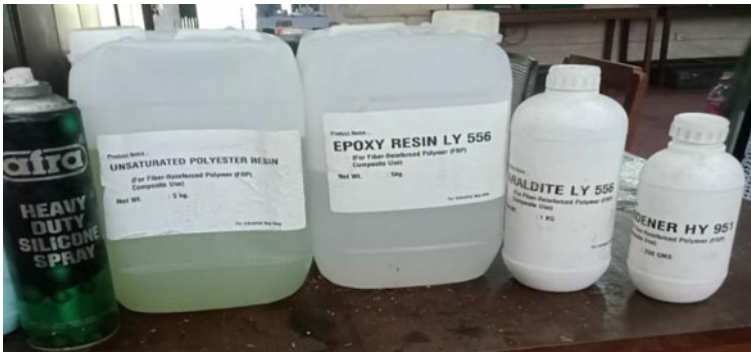
Fig. 2 Raw materials—epoxy, hardener and silicone spray
