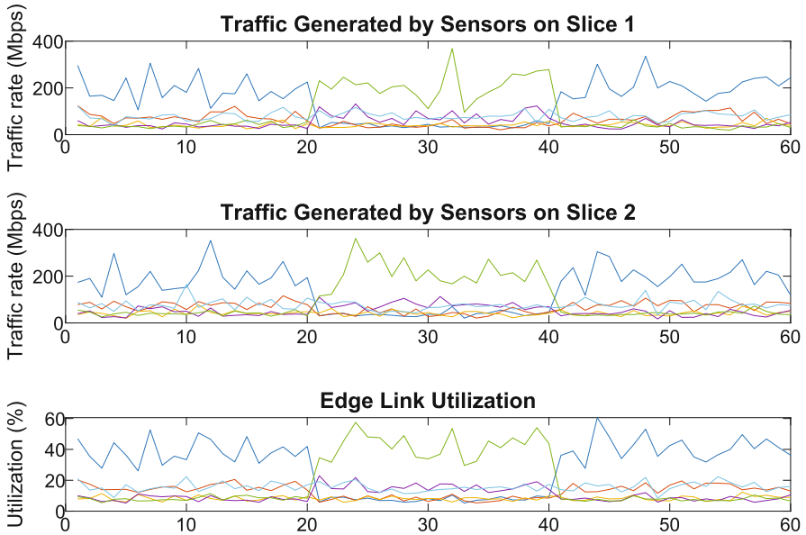
Fig. 6.5 The rate of traffic generated by sensors and the resulting edge link utilization. The x -axis represents the iteration number
