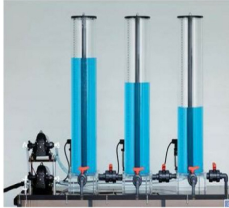
Fig. 4. Three tank of TTS20
