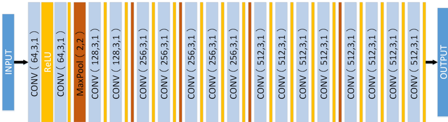
Fig. 4. VGG network. Network with corresponding kernel size, number of feature maps and stride indicated for each convolutional.
