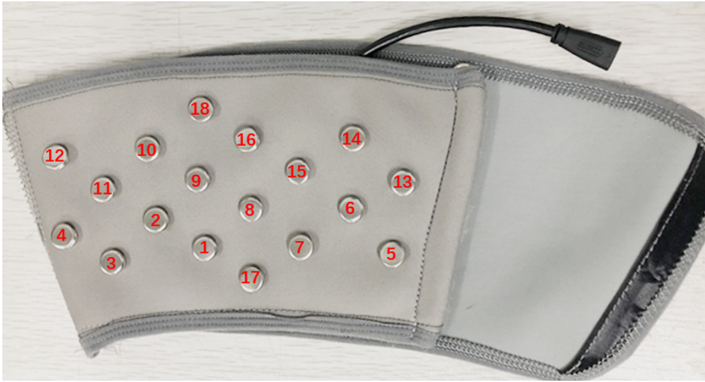
Fig. 2. The electrode sleeve for sEMG signal recording, 16 monopolar channels record the differential voltage between electrode 1–16 and electrode 17 and 18 provides the bias voltage to remove DC offset.
