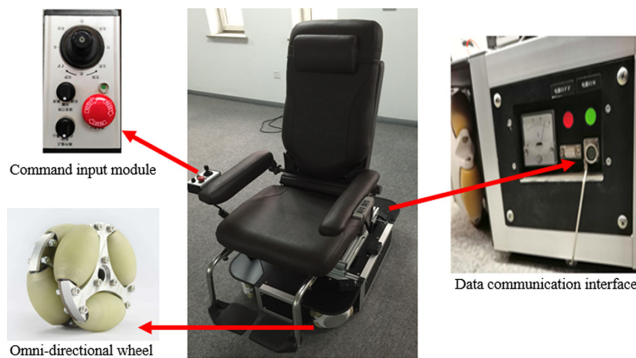
Fig. 1. The function and structure of the intelligent wheelchair
