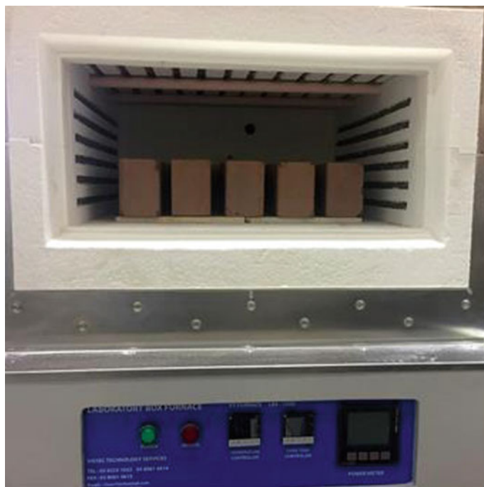
Fig. 2 Selected brick samples were positioned vertically to ensure even firing in a furnace
