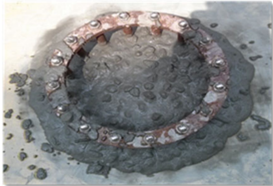
Fig. 3 Passing ability of FA and BA incorporated in SCC using the J-Ring test
