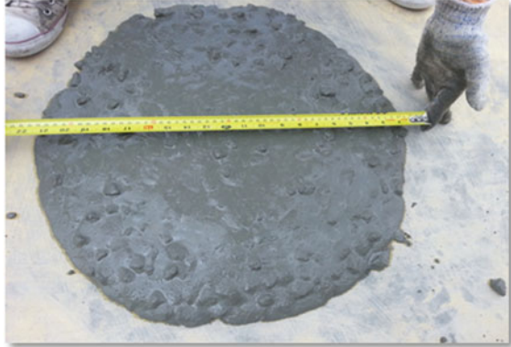
Fig. 2 Slump flow of FA and BA incorporated in SCC using t500 test
