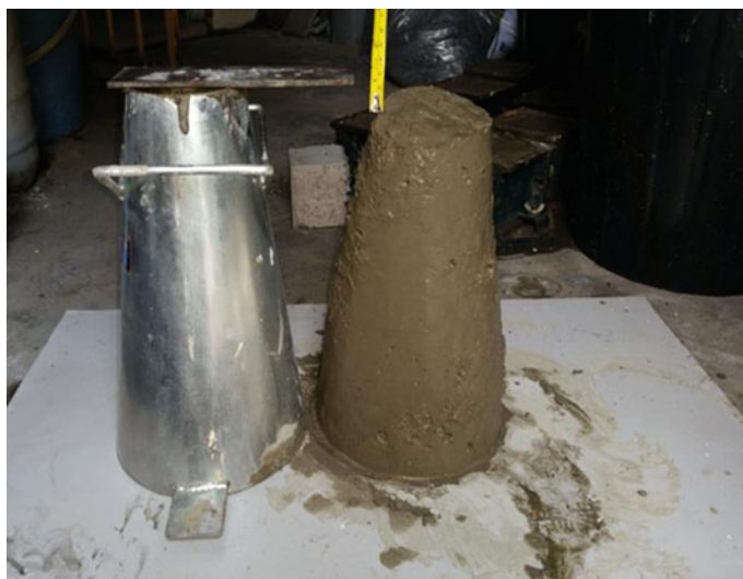
Fig. 8 The slump test for concrete incorporating sintered geopolymer volcanic ash artificial lightweight aggregate (SGVA)
