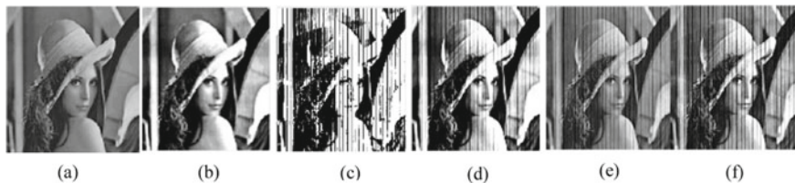
Fig. 3 Image compression results for a exact multiplier b multiplier 1, PSNR = 14.882 c multiplier 2, PSNR = 8.3581 d multiplier 3, PSNR = 12.881 e multiplier 4, PSNR = 20.1896 and f multiplier 5, PSNR = 15.3463
