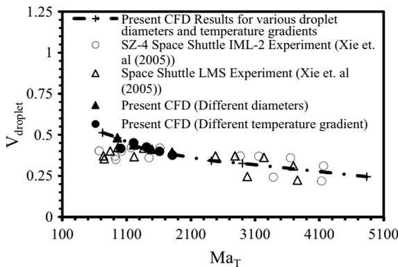
**Fig. 1** Validation of present CFD with experimental data
