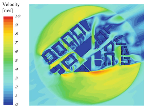
Fig. 3 Velocity contour at pedestrian level of 2 m using realizable k-\epsilon model, wind direction: 240^\circ
