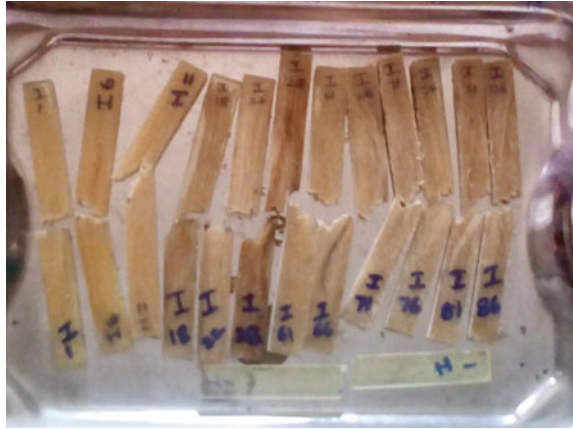
Fig. 19 Impact fractured type 1, 2, 3 and 4 and composition 1, 2, and 3 epoxy composite specimens
