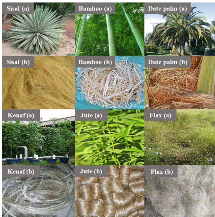
Fig. 1 Different types of plants (a) and their extracted fibers (b) (Shridhar 2019; Kiasif 2018; Hakeeml et al. 2014; Ferreira et al. 2017; Suzuki and Arai 2015; Gondal et al. 2018; Goudenhooff et al. 2019; Gondall et al. 2018; Abdul Ajeez 2017)
