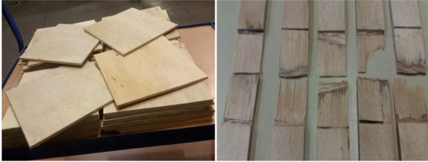
Fig. 7 Manufactured plywood by Soy based adhesive (Ghahri et al. 2017)
