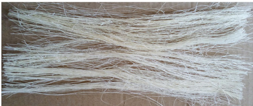
Fig. 1 Agave Americana fibre after oven drying, cutting
