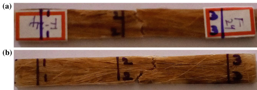
Fig. 2 Measurement of specimen dimensions at different sections, a flexural; b impact
