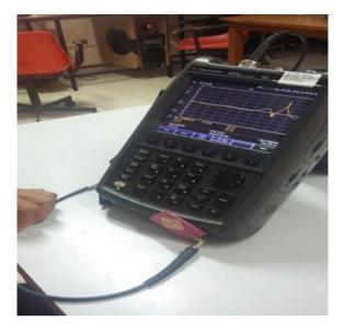
Fig. 11 Testing of antenna using vector network analyzer
