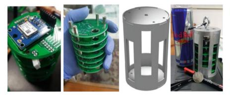
Fig. 12 Final assembly of CanSat
