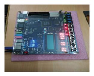
**Fig. 14** Hardware implementation of proposed DRPPG-based reconfigurable DA FIR filter in ALTERA FPGA
