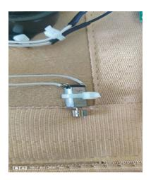
vibration motor helps in providing the vibration alert to the user who wear this jacket (Fig. 2).
