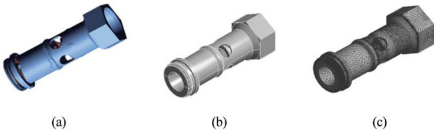
Fig. 1 Schematic of oil tank injector, a real injector, b 3D model in CATIA, c meshing model in ANSYS
