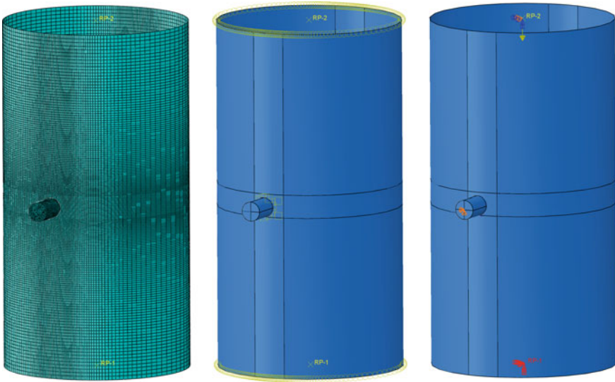
Fig. 4 Numerical modeling of the axial compression and poking
