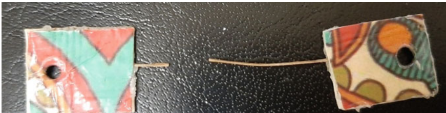
Fig. 5 Test specimen after breaking of the fiber
