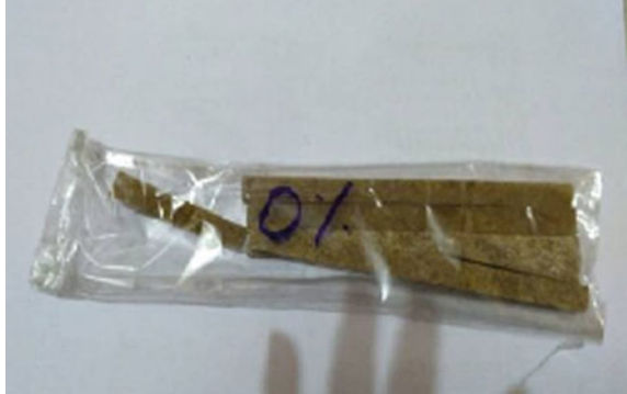
Fig. 5 C1 specimens with epoxy & 20 wt% sugarcane trash
