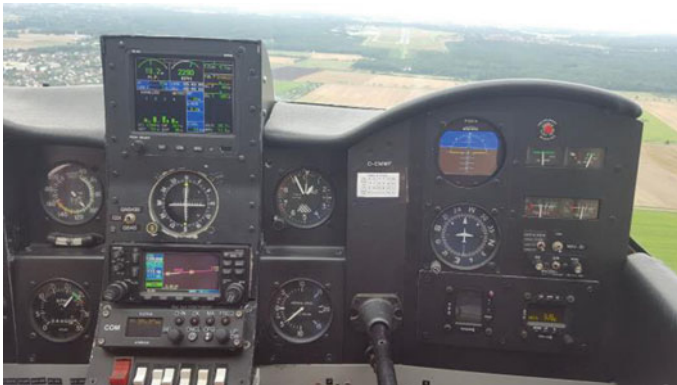
Fig. 2 Cockpit of cessna 172N
