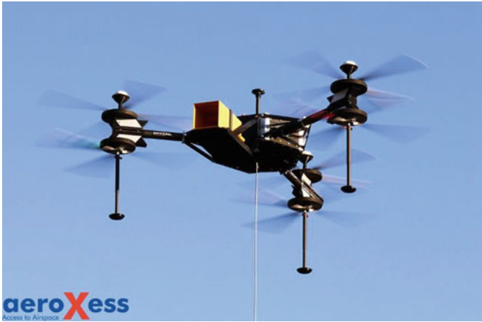
Fig. 5. H1-UAV equipped with L-band probe antenna and 6D-RTK equipment
