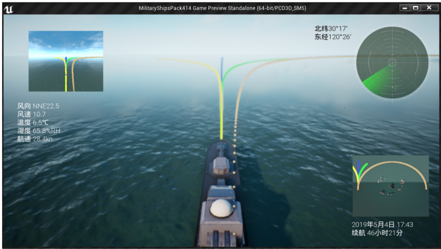
Fig. 4. Immersive unmanned boat remote control system interface implemented by UE4 game engine
