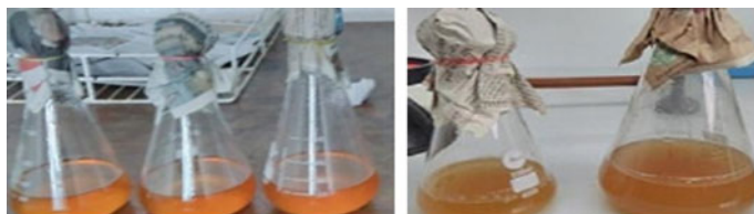
Fig. 3 Prepared broth for concrete with bacteria
