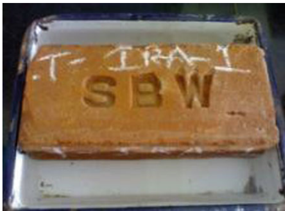
Fig. 5 Water absorption test on brick
