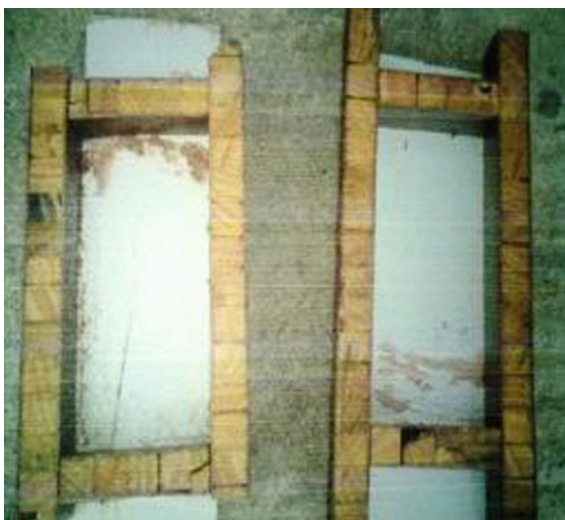
Fig. 2 Mold preparation for brick casting
