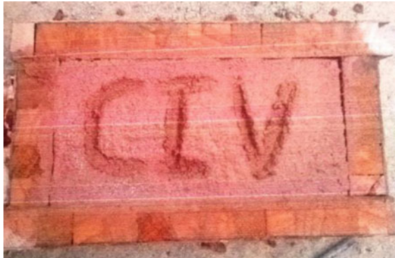
Fig. 4 Sample brick casted in laboratory conditions
