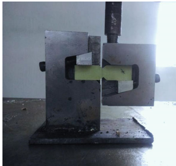
Fig. 4 Iosipescu shear test fixture
