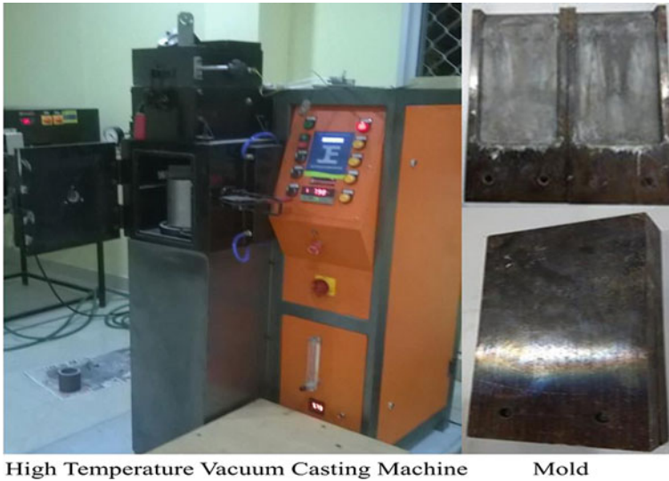
Fig. 11.1 High-temperature vacuum casting machine and cast iron mold
