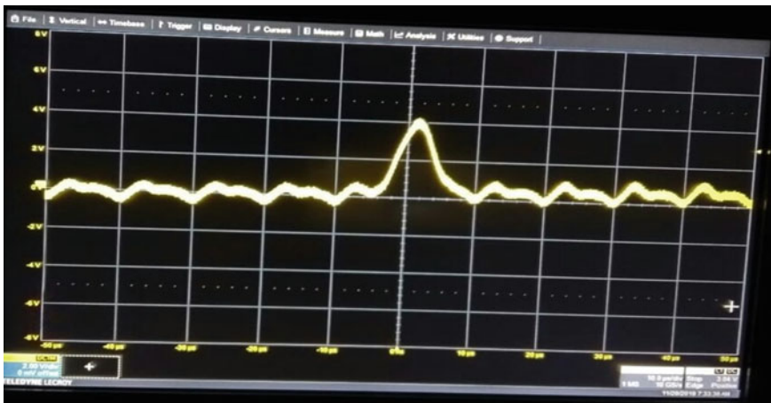
Fig. 175.4 Signal with Fe^{55} source after spectroscopic amplifier Gain = 50, Shaping time = 2 \mu s)
