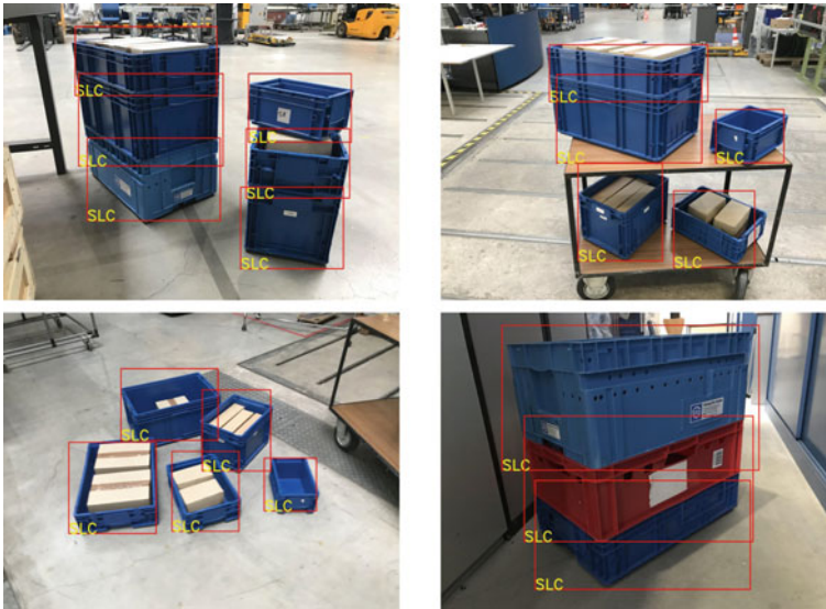
Fig. 1 Prediction results of a fully-synthetic trained object detector. The detection model is trained on synthetic image data only using the proposed image generation approach. To meet industrial requirements, we implement novel features to represent specific object relations, to suppress false detections and to model complex industrial lighting conditions while maintaining a maximum level of scalability
