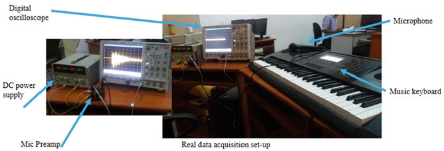
Fig. 7 Real data acquisition setup
