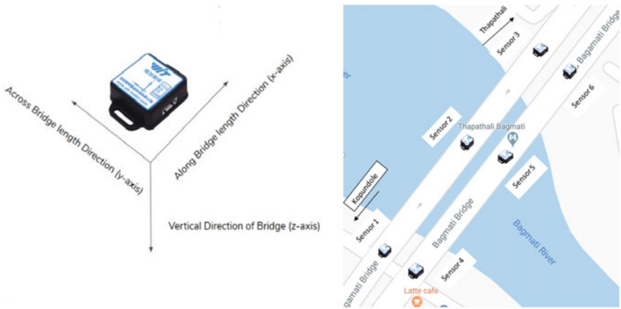
Fig. 4 Illustration of Sensors installation in the Thapathali–Kupondole bridge
