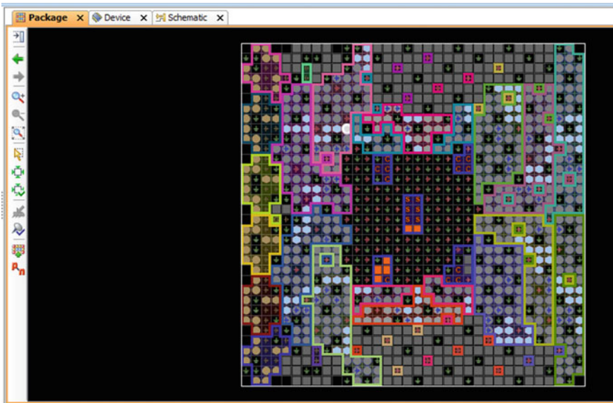
Fig. 18 Package schematic of Wallace tree 8 * 8 multiplier
