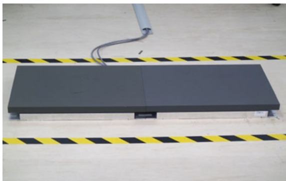
Fig. 4 2-tile pressure plate by Qualisys
