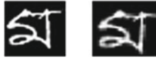
Fig. 8 Original image (left) and augmented image (right) with rotation = 10°, zoom range = 0.1, height and width shift range = 0.1
