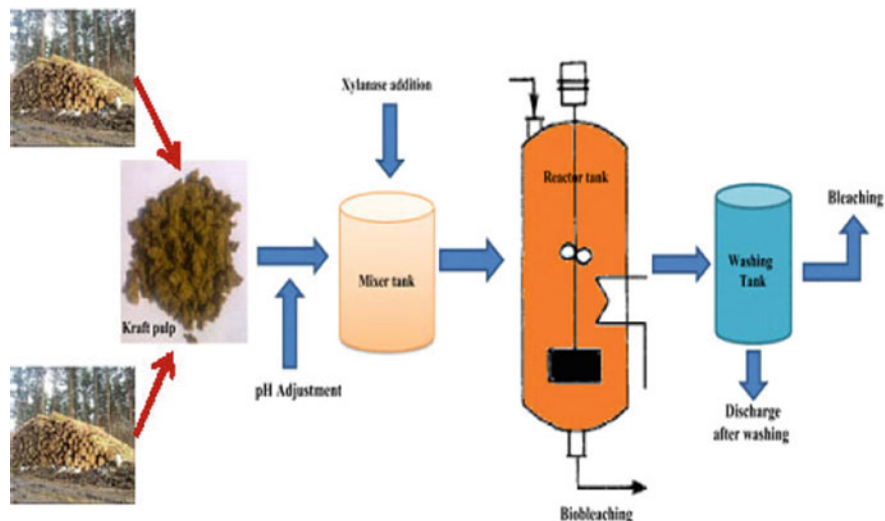
Fig. 16.7 General flow-diagram of biobleaching process (Kumar et al. 2016)
