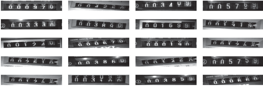
Fig. 4. Carry data set. The meter ends with 0 and 9 is in carrying state. The ratio of the figure is on purpose to make the deep learning model more robust. There might be some slope angle on images' views.
