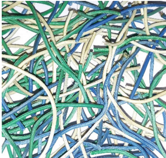
Fig. 9 PVC-insulated waste copper wires
