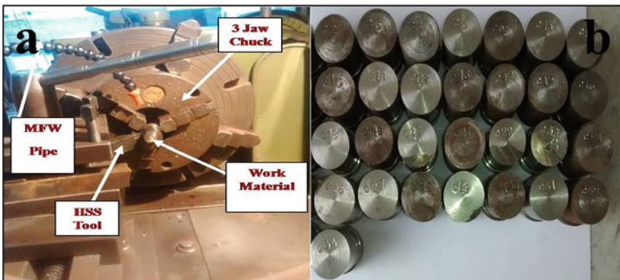
Fig. 2 a Experimental setup for carrying out turning operation, b machined samples
