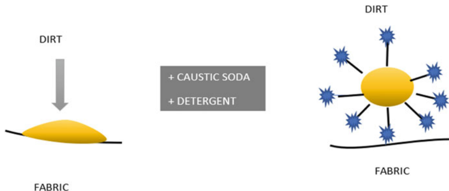
Fig. 18.6 Conventional scouring process
