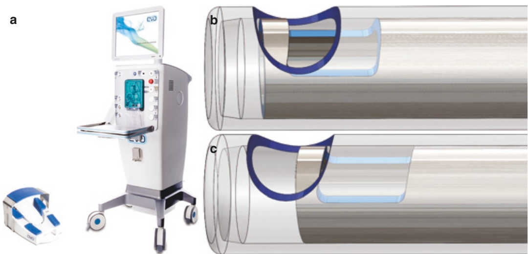
Fig. 5.4 (a) EVA vitrectomy system. (b and c) Vitreous cutter with two dimensional cutting with another port in the inner shaft (Image courtesy of DORC)
