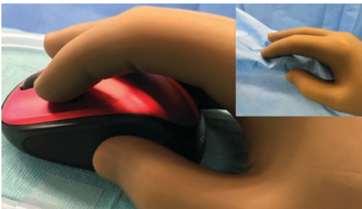
Fig. 9.5 Wireless computer mouse on the armrest of the operating chair used under a sterile surgical draping
