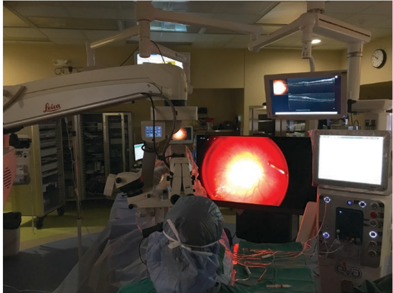
Fig. 3.5 Modern vitreoretinal surgery intraoperative theater. Vitrectomy surgical platform, Heads-up 3D visualization system, Leica Enfocus intraoperative OCT system on Proveo 8 microscope
