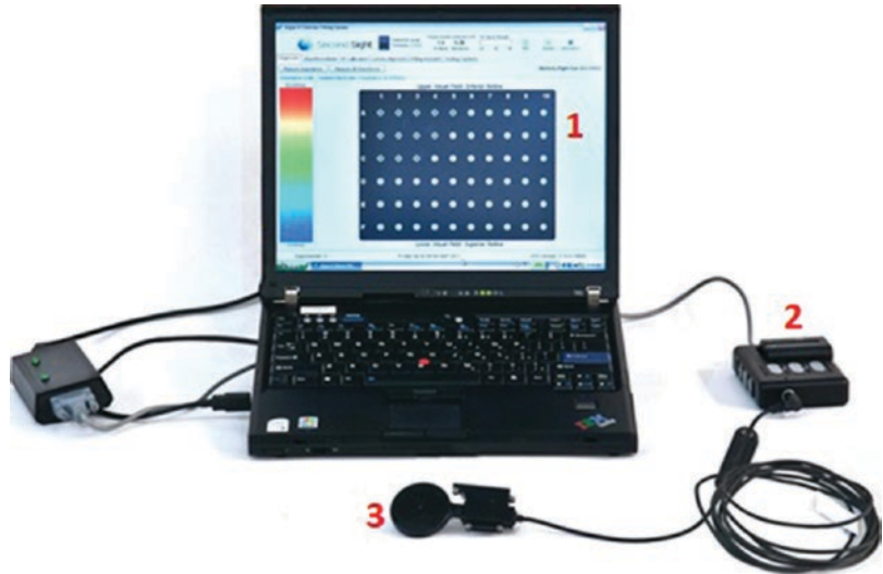
Fig. 41.5 Intraoperative impedance test equipment (1) CFS Laptop with dedicated software; (2) VPU; (3) OR coil
