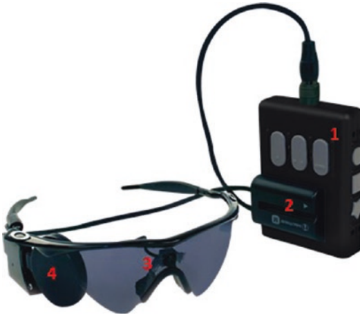
Fig. 41.3 (1) Video processing unit (VPU); (2) battery; (3) glasses with the central camera; (4) receiving coil
