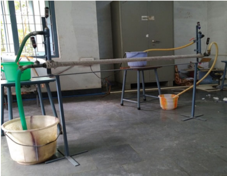
Fig. 1 Experimental setup-photographic view (tube-in-tube heat exchanger)
