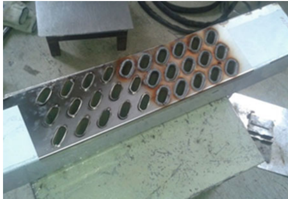
Fig. 2 Fabricated laser cut SS304 metal sheet of crossflow heat exchanger
