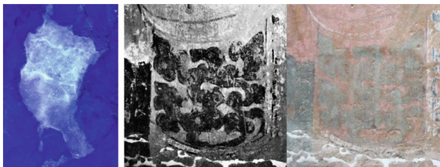
Fig. 15.21 The optical investigation using UV fluorescence helped identify the presence of the reinforcing gypsum repairs
