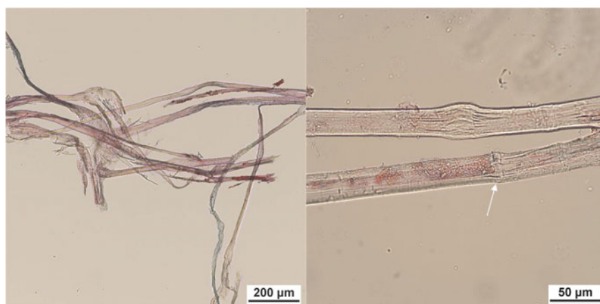
Fig. 15.9 Microscopic examination of fibres from the finishing plaster layer (left: dissociated fibre, right: fibre node)
