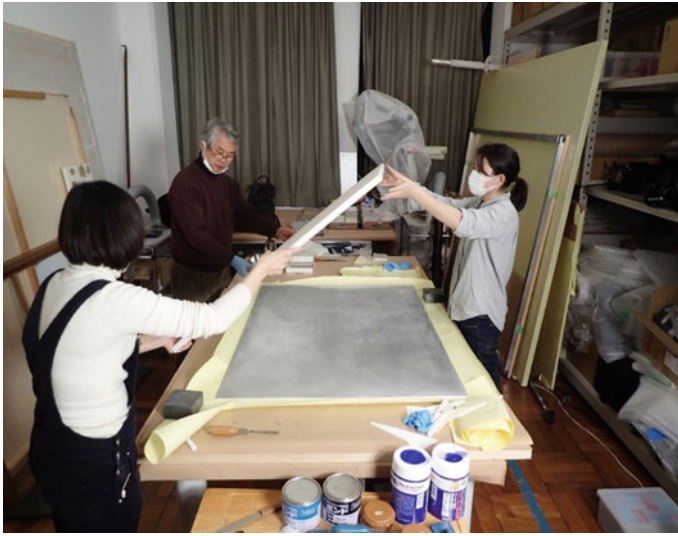
Fig. 11.18 Adhering ROHACELL on to the aluminum board
