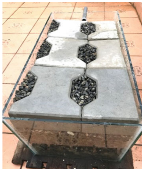
Fig. 2 Structure of the pervious pavement experimental setup
