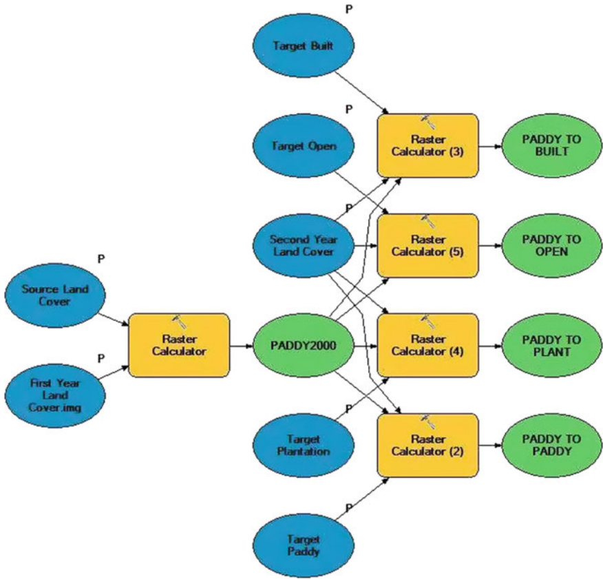
Fig. 3 ArcGIS model for calculating transitions of agricultural land to other land uses
